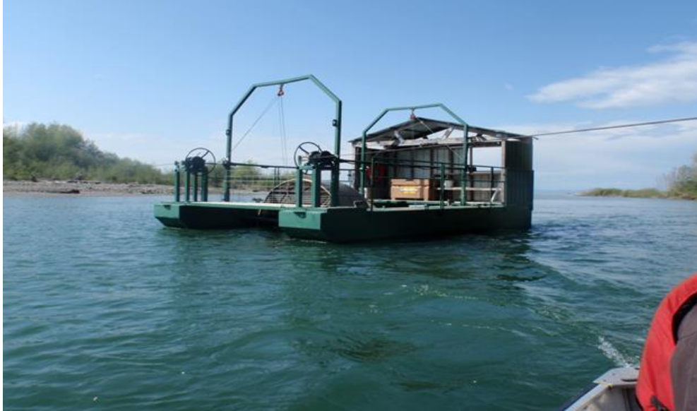
Figure 2. Top Elwha River 8' rotary screw trap fishing at Rkm 0.3 during the pre-dam and post-dam removal periods and bottom 5' rotary screw trap used during dam removal.
